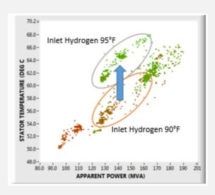
A PD monitoring system applied to a 200 MVA turbo-generator highlighted an inverse relation between PD activity and the machine temperature. Simply acting on the temperature regulator of the cooling hydrogen it was possible to avoid the stator core temperature to decrease below 59°C, defined as the boundary for acceptable PD level from the PDE Map. During the following weeks, the machine was operated in the same load range, but with a different regulation of the inlet hydrogen
