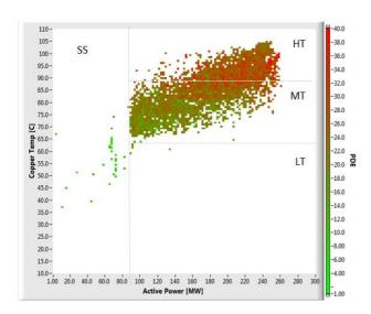
Looking at the beside Map, obtained from 300 MVAVPI Turbo-Generator, а concentrations of red dots are mainly occurring in the HT zone, which means at High Temperature. It is also clear that the red dots are occurring at any power level between 140 and 300 MW, which means that the PD mechanism is not directly dependent on load. As a matter of facts, red dots clearly start to occur above 85°C. This behaviour indicates the presence of degradation at the semi-conductive
