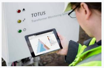
Ability to perform Duval's triangle, and access live data from any smart device
